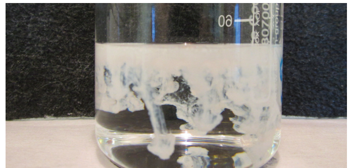
Fig. 3: Clearstrength® XT100 spontaneous dispersion into MMA monomer, without shear
